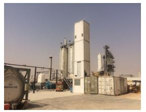
Ooms PMB installed and operated a mobile Sealoflex<sup>®</sup> PMB blending plant at the project site, processed the 60/70 bitumen to the required PMB specification and discharged it to the bitumen tanks of the asphalt batching plants of its client (just in time principle).
